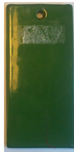
HR60® Extra G (Green) without cut AFTER testing
